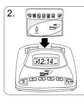
Install the alarm clock or trickle charger (Part no's. CH3A-2205-IN, TR3A-2206-EU), insert the Pager into the charging slot and charge for 24 hours.
