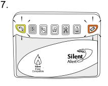
If the low battery sequence alternates with another event key, that monitor has a low battery.
